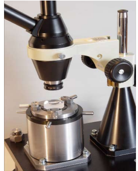
Technological device for central sticking and mounting optical components
