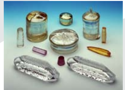
Oxide single crystals, Single crystal substrates for HTSc layers, Quartz and SAW substrates
