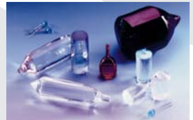
Substrate materials for GaN – blue optoelectronics, Neodymium gallate, sapphire, mixed perovskite (La, Sr)(Al, Ta)O 3 (LSAT)
