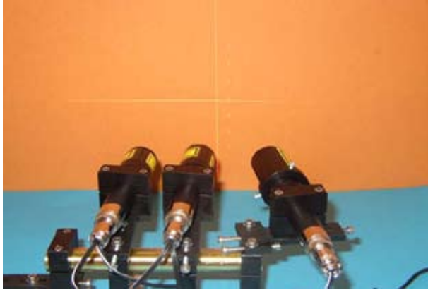
EXAMPLE OF A THREE LASER MODULE ASSEMBLY ALONG WITH MOUNTING ELEMENTS.
